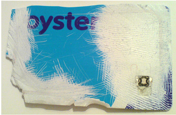
A damaged card, revealing the microchip in the lower right corner and the aerial running around the edge of the card.
