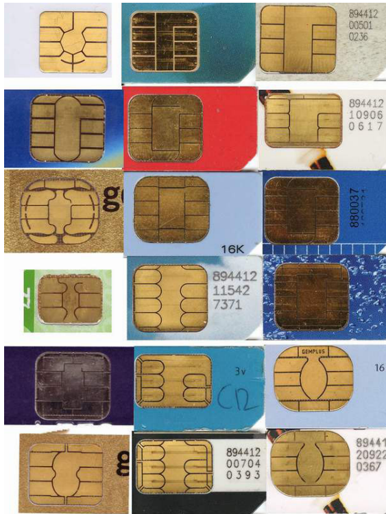
Contact-type smart cards may have many different contact pad layouts, such as these SIMs
